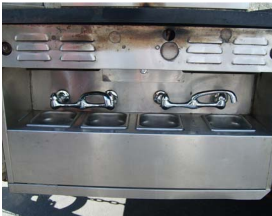
An example of a three compartment sink and a handsink on a pushcart.
